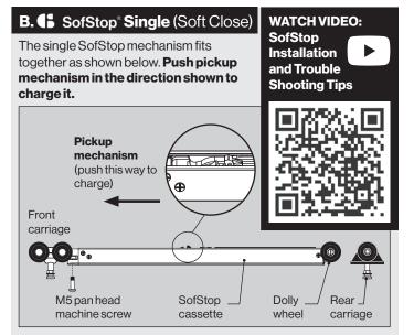
To load the SofStop mechanism into the track:
