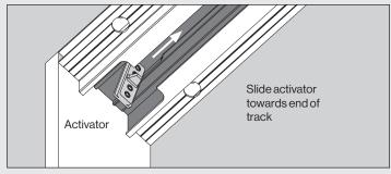
Insert the rear carriage, cassette and front carriage using the same method as Single Sofstop (B). Secure the carriage to the cassette.
