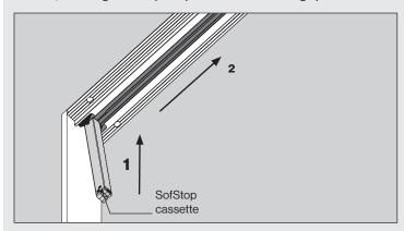
Slide the front carriage into the track with the tow bar facing into the pocket.
