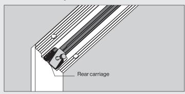
b) Insert the cassette into the notched end of the track, dolly wheel first, ensuring that the pickup mechanism is facing up.
