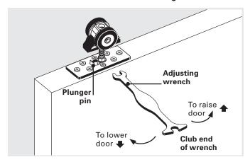
Note: The top of the hanger shaft screws into a self-locking nut. If the hexagonal nut is turned downwards too far, the shaft will become loose from the self-locking nut. If the turning resistance suddenly feels much easier, you have gone too far.
